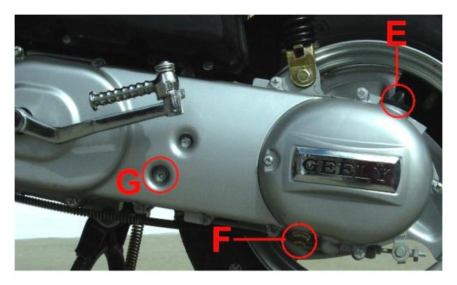
The filler hole is marked "E" in the picture below. The drain plug is marked "F". The screw marked "G" is the safety filler screw. Remove this screw while re-filling the oil and you will be sure not to trash your clutch. The oil will simply drain out of this hole before getting too high and touching the clutch.
