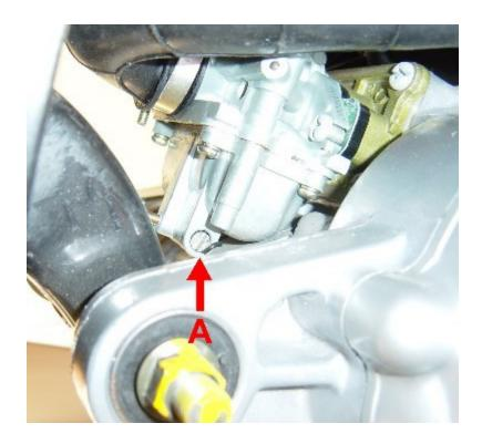
The fuel leak mentioned above is in reference to the VENT connector on the vacuum operated fuel valve. On the Retro and FX16 models, this connector is not used. Geely blocks it off with a short hose plugged with a screw. Sometimes, these begin to leak fuel, which presents a safety hazard. The best way to seal the leak is to replace the screw with a 1/4" Ball Bearing followed with a small clamp to hold it into place.
